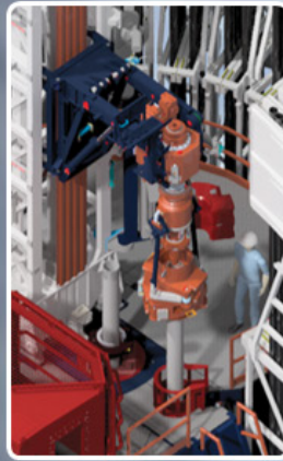
Top drive dolly extended to reach mouse hole
